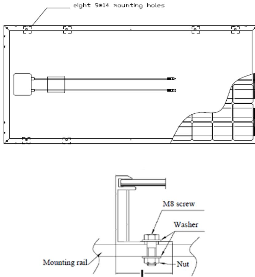
Figure 2: PV module installed with Screw fitting method
